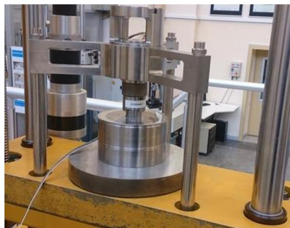
Figure 7: Calibration of a 10 kN transducer on the 20 kN PTB D-FSM
