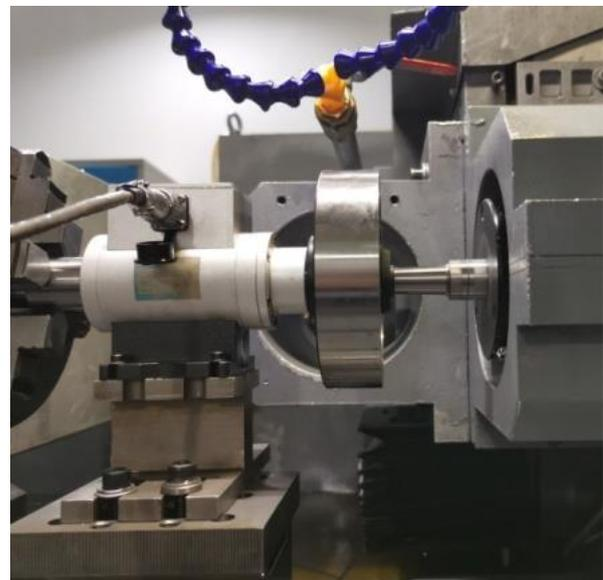
Figure 2: Experimental assembly for measurement based on standard torque sensor
