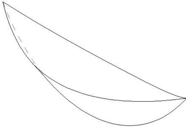
Figure 7: Shape of contact area in internal thread grinding process
