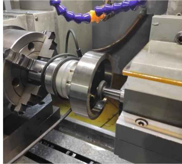
Figure 1: Experimental assembly for measurement based on six-axis torque sensors
