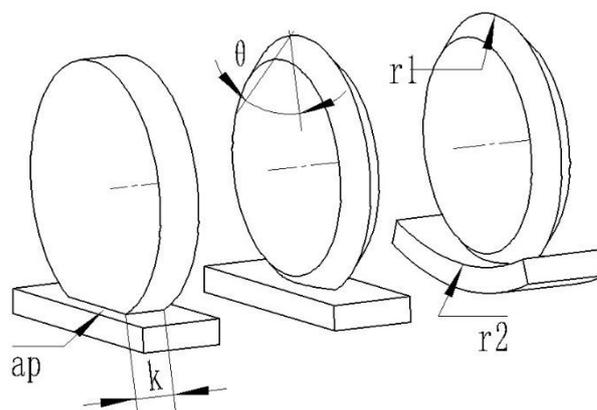
Figure 4: The instantaneous contact models of flat grinding, flat groove grinding and internal thread grinding
