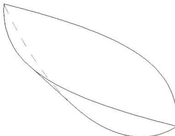
Figure 6: Shape of contact area in flat groove grinding process
