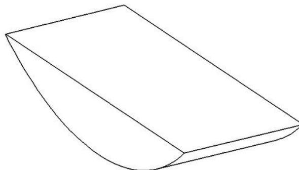
Figure 5: Shape of contact area in flat grinding process
