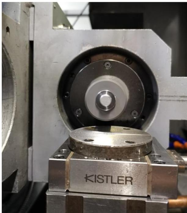
Figure 3: Experimental assembly for measurement based on three component dynamometers
