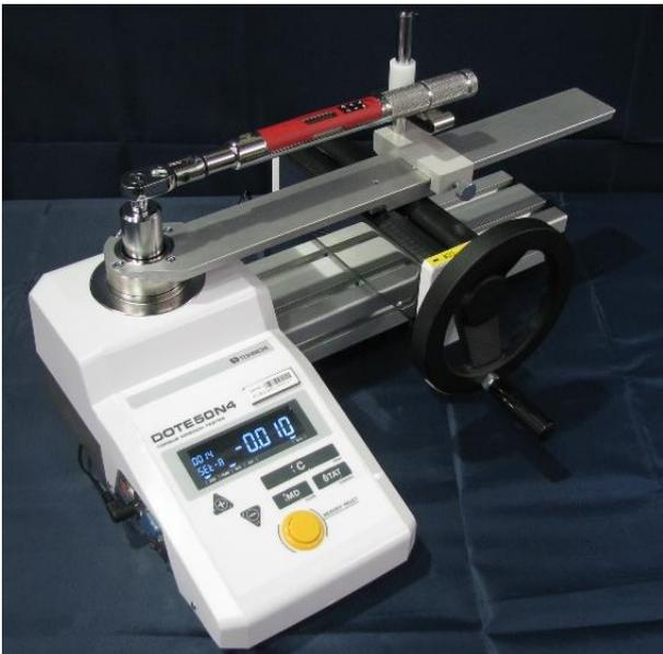
Figure 2: The torque wrench tester (TWT) used as a reference standard
