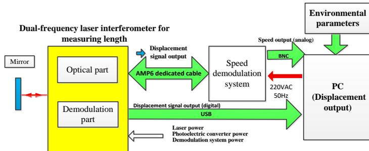
Figure 4: Scheme diagram of dual-frequency heterodyne laser interferometer system
