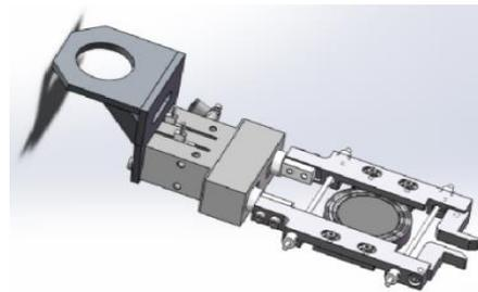
Figure 7: Schematic diagram of gripper
