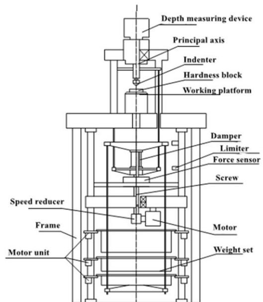
Figure 3: Rockwell hardness measuring device
