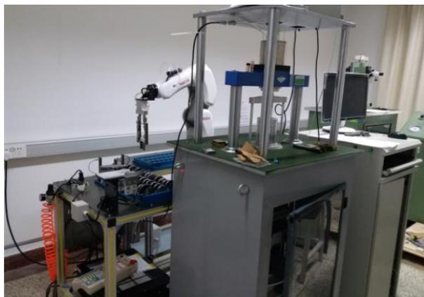
Figure12: Unmanned precision measurement and calibration device for Rockwell hardness
