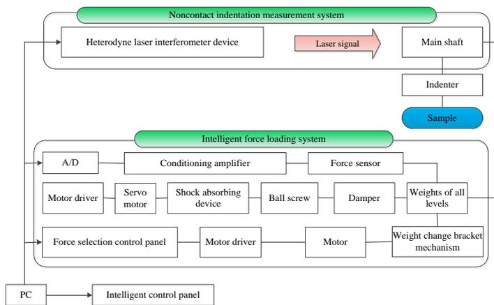
Figure 2: Overall structure diagram of intelligent loading laser Rockwell Hardness standard device
