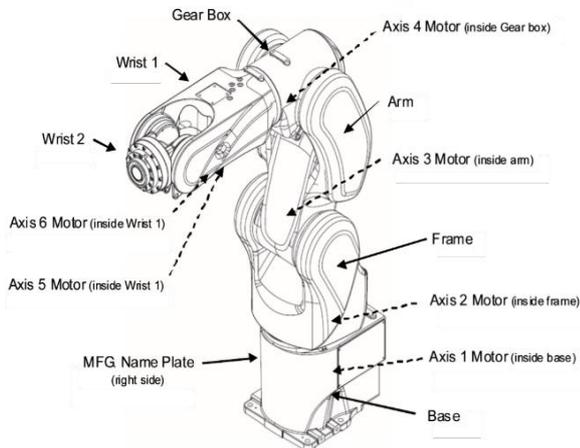
Figure 5: Mz04-01 Robot body appearance diagram
