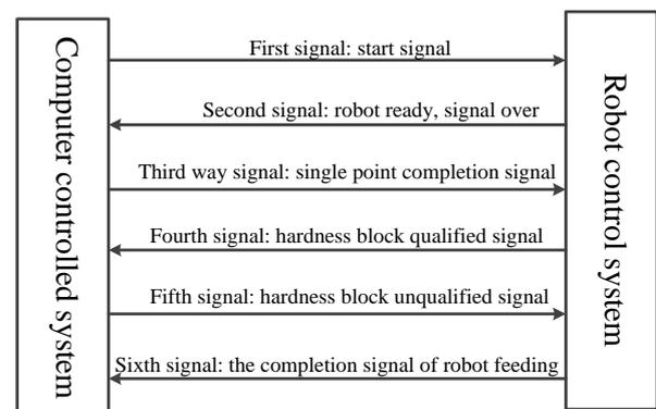
Figure 11: Interaction signals between computer and robot
