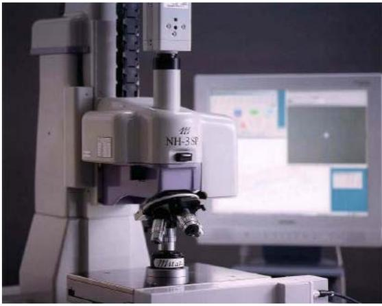
Figure 1. The laser probe 3D profile measurement instrument used to measure the cross section of Rockwell diamond indenters (courtesy of Mitaka Koki, Co. Ltd.).
