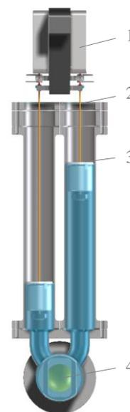
Figure 1: U-tube main assembly consisting of the differential interferometers (1), viewports (2), pool floats (3) and the density standard (4).
