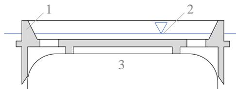
Figure 4: Pool float setup consisting of the PTFE pool float (1), free surface of the vacuum oil (2) and buoyancy body (3).
