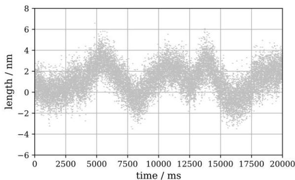
Figure 3: Length signal of a differential interferometer, when the measurement beam is reflected from the vacuum oil's surface, recorded with a sampling rate of 1 kHz.
