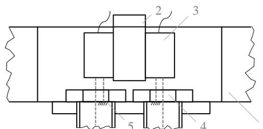
Figure 2: Interferometer setup containing the granite structure (1), stainless steel interferometer carrier (2), differential interferometers (3), viewports (4), reflective coating (5).
