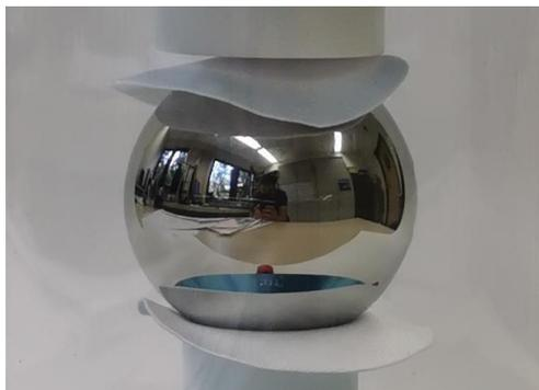
Figure 5: PTB's titanium density standard DS1, owning a nominal volume of 100 cm<sup>3</sup>.
