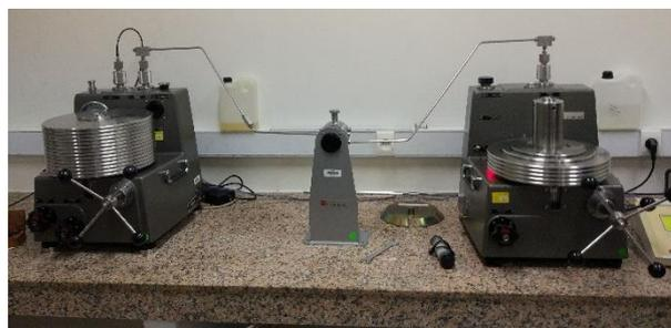
Figure 1: Setup used for the determination of the piston-cylinder effective area. The reference pressure balance, on the left, is working with gas and the pressure balance under calibration, on the right, is working with oil.
