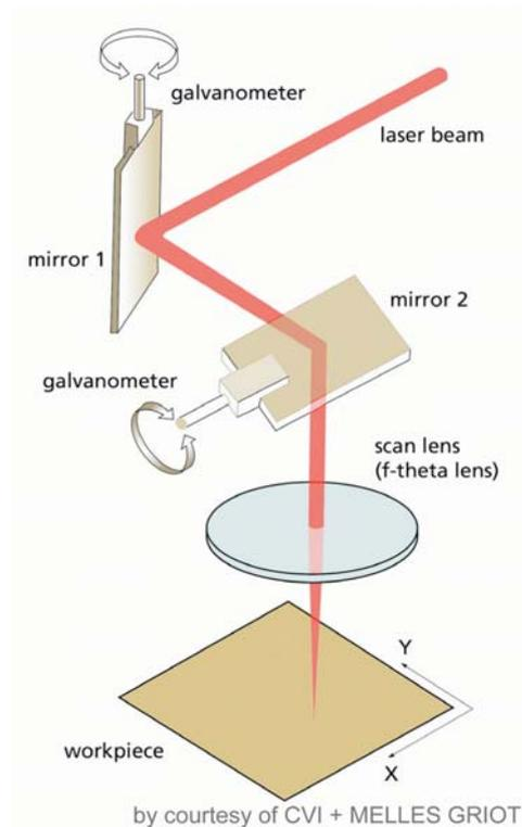
Fig. 2: Scheme of a galvanometer-driven scanner [4]
