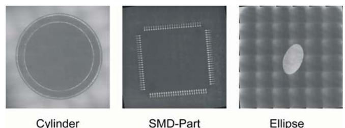
Fig. 5: Stitched images used for evaluating the accuracy in position estimation
