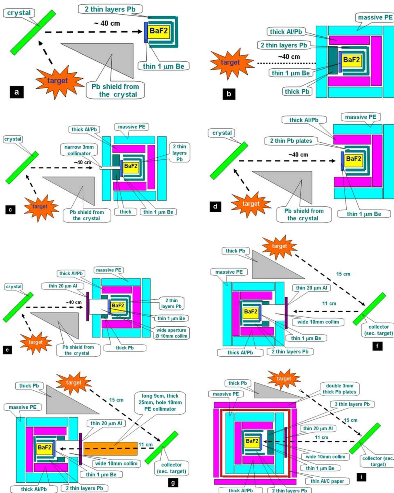
Fig. 8: Schematic illustration of the target and shield setups investigated for the BaF<sub>2</sub> detector. The geometric setup is determined by the position of the primary target, the (eventual) crystal/collector as a secondary target, and the detector. The shield assembly was composed of materials with polyethylene (PE), lead (Pb), Aluminum (Al), a thin Beryllium (Be) foil window in various segment sizes and thicknesses
