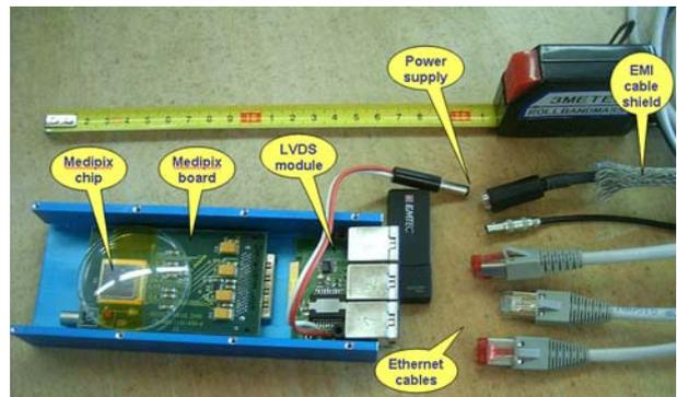
Fig. 3: Medipix2 detector and LVDS Module with communication ethernet and power cables. The EMI shield for one cable is shown
