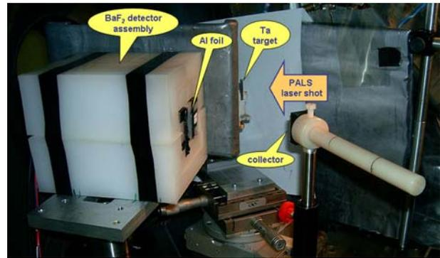
Fig. 7: Indirect experimental setup in the PALS interaction chamber: The BaF<sub>2</sub> detector assembly, facing the secondary target – the collector, is shielded from the primary Ta target
