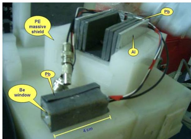
Fig. 4: BaF<sub>2</sub> detector with lead (Pb), Aluminum (Al) and Polyethylene (PE) shield
