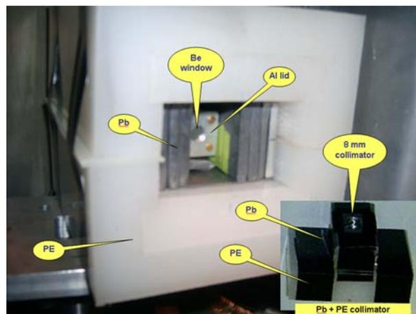
Fig. 5: Shield assembly for BaF<sub>2</sub> detector with lead (Pb), Aluminum (Al) and Polyethylene (PE) segments. The Pb/PE shield with 8 mm collimator is shown in the inset
