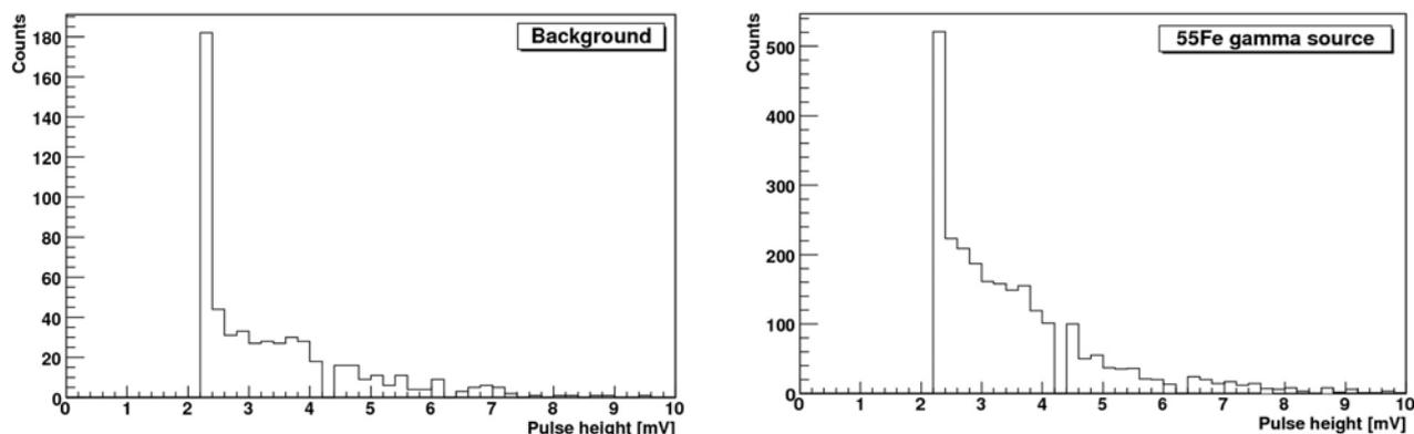
Fig. 2: Amplitude spectra of background (left) and  $^{55}\text{Fe}$  source (right) collected with the  $\text{BaF}_2$  detector
