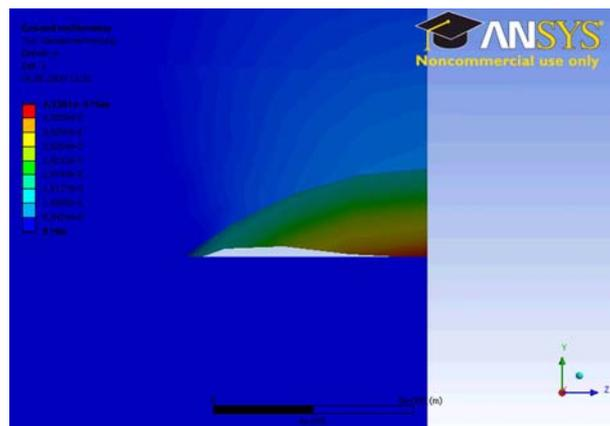
Fig. 15: ANSYS simulation of valve type 3 in the closed state when actuated with 0.5 bar in the pneumatic layer. Perspective from inside the channel
