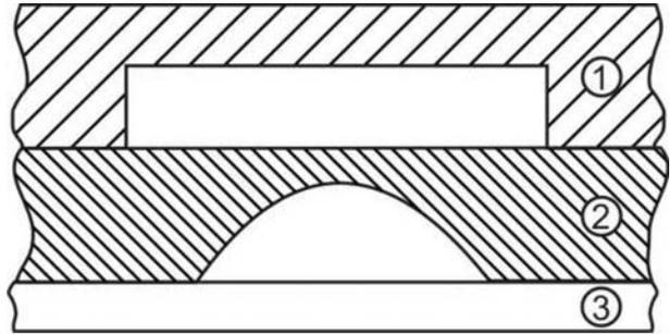
Fig. 4: Valve type 3. Cross-section of valve area with round channel geometry. 1: pneumatic layer; 2: fluidic layer; 3: substrate
