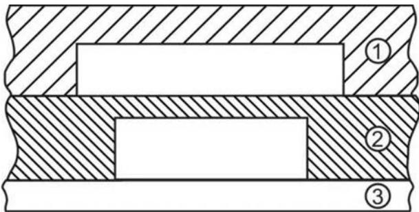
Fig. 3: Valve type 2. Cross-section of valve area with rectangular channel geometry. 1: pneumatic layer; 2: fluidic layer; 3: substrate
