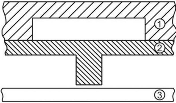
Fig. 2: Valve type 1. Cross-section of valve area with interrupted fluidic channel. 1: pneumatic layer; 2: fluidic layer; 3: substrate
