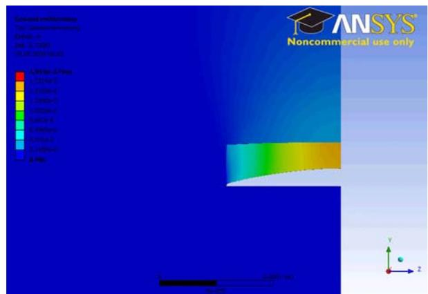
Fig. 11: ANSYS simulation of valve type 1 in the opened state when actuated with negative pressure of 0.2 bar in the pneumatic layer. Perspective from inside the channel
