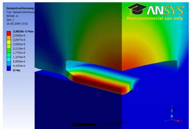
Fig. 12: ANSYS simulation of valve type 2 in the closed state when actuated with 0.5 bar in the pneumatic layer
