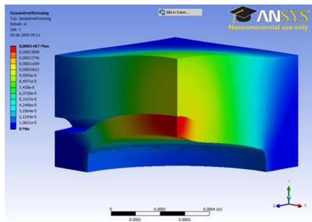
Fig. 16: ANSYS simulation of valve type 4 in the closed state when actuated with 0.75 bar in the pneumatic layer
