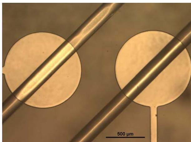
Fig. 7: Pneumatically actuated valves over fluid channels
