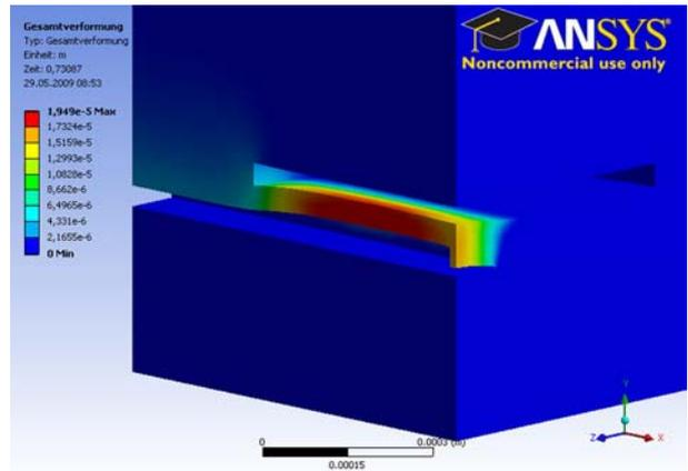
Fig. 10: ANSYS simulation of valve type 1 in the opened state when actuated with a negative pressure of 0.2 bar in the pneumatic layer
