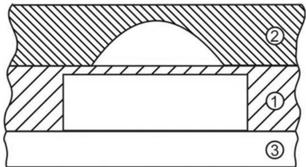
Fig. 5: Valve type 4. Cross-section of valve area with round channel geometry. 1: pneumatic layer; 2: fluidic layer; 3: substrate
