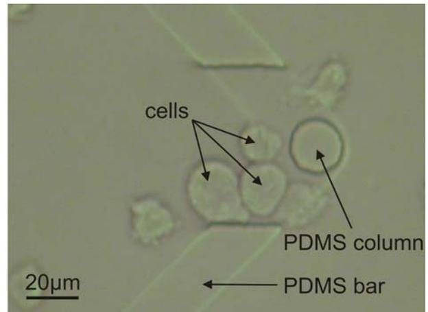
Fig. 17: Cell accumulation in the reaction chamber
