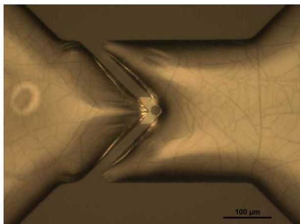
Fig. 9: Reaction chamber. Cells can be accumulated in the central structure
