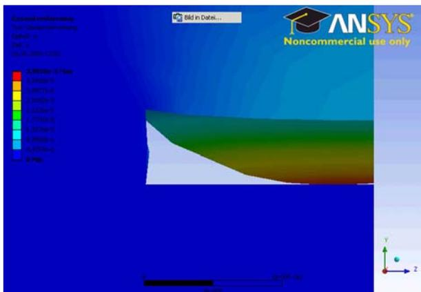
Fig. 13: ANSYS simulation of valve type 2 in the closed state when actuated with 0.5 bar in the pneumatic layer. Perspective from inside the channel
