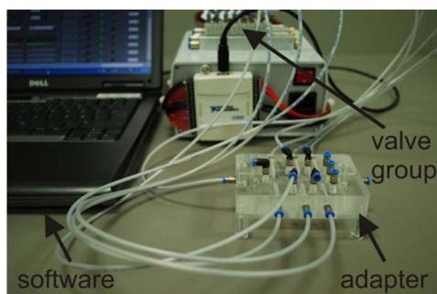
Fig. 8: Experimental setup with a microfluidic chip mounted on an adapter. The adapter is pneumatically connected via a centralized and software-controlled valve group
