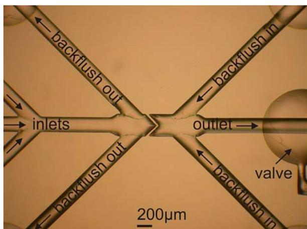
Fig. 6: Microfluidic network with inlet and outlet channels, backflush channels and pneumatic valves
