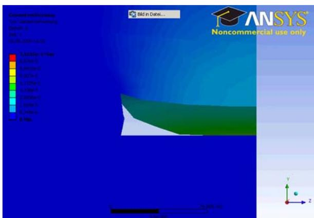
Fig. 14: ANSYS simulation of valve type 2 in the closed state when actuated with 1.0 bar in the pneumatic layer. Perspective from inside the channel
