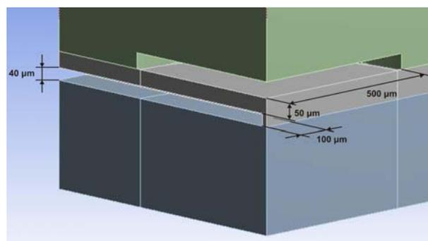
Fig. 1: Common geometrical parameters of all valve types
