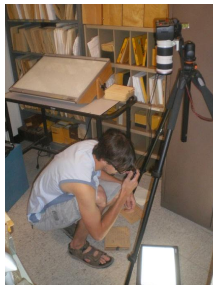
FIGURE 1. Digitizing plates with a transportable device in the plate vault of the Steward Observatory, Tucson, AZ. This digitization technique can be used even in very small rooms.
