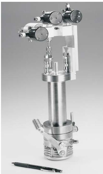
Fig. 4: Photograph of the pressure gas target
