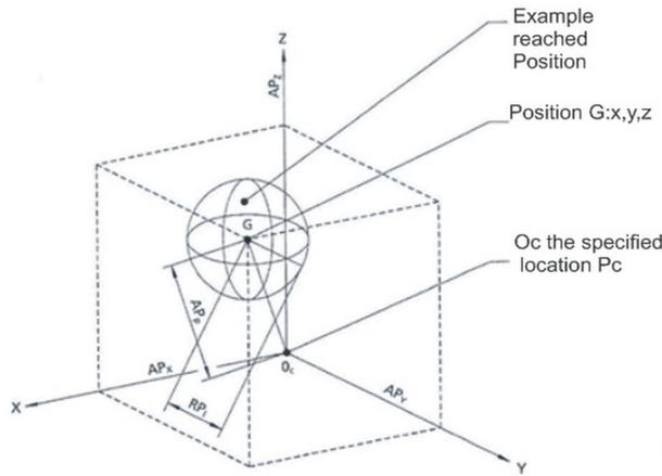
FIGURE 5. Unidirectional positioning accuracy.
