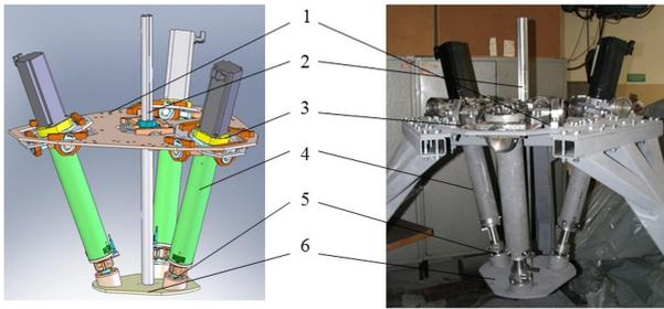
FIGURE 1. A computer model and a real model of Tricept: 1–solid platform, 2–central pole, 3–universal (primary) joint, 4–telescopic pole, 5–spherical (secondary) joint, 6–movable platform.
