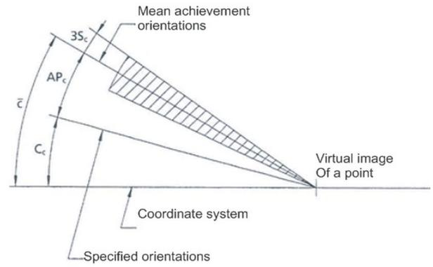
FIGURE 6. Unidirectional orientation accuracy.
