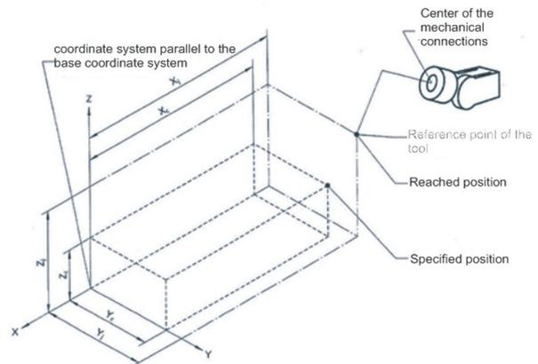
FIGURE 4. The relationship between the specified position and the reached position.
