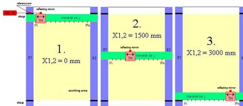
FIGURE 4. Scheme of measurement axes Y.
