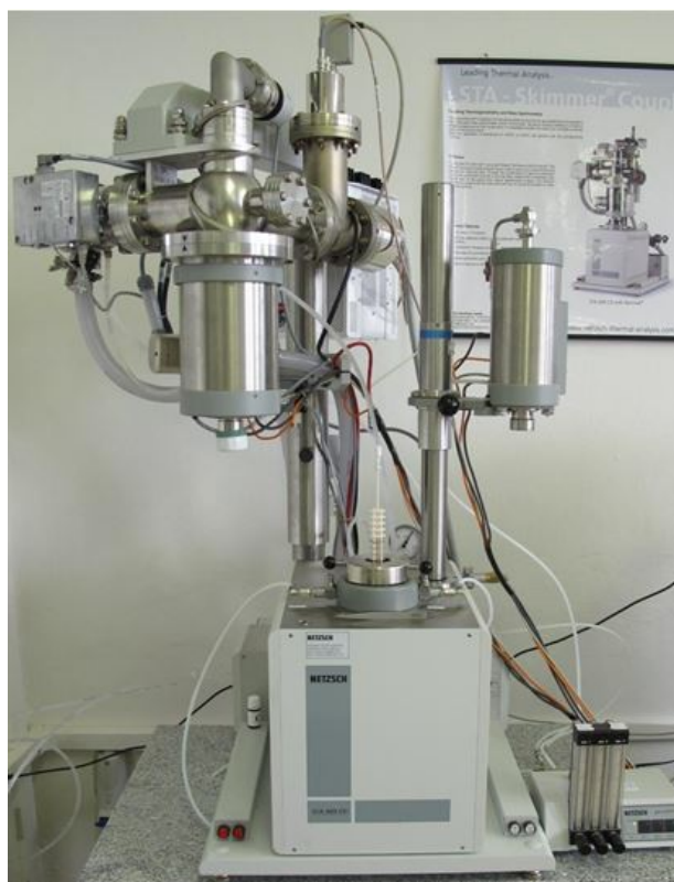
FIGURE 1. Netzsch STA 409CD — Simultaneous Thermal Analysis Apparatus.
