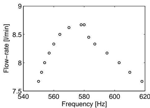
FIGURE 10. Frequency characteristic of the air volume flow-rate at input voltage  $|U_{in}| = 15$  V with the hose clamp removed.
