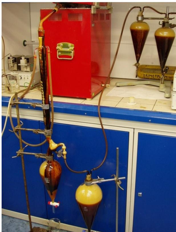
FIGURE 1. Pyrolysis apparatus: 1–furnace, 2–water cooler, 3–separators, 4–sampling bag or gas burner.
