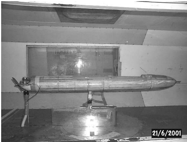
Fig. 14: Fuselage installed in the tunnel
