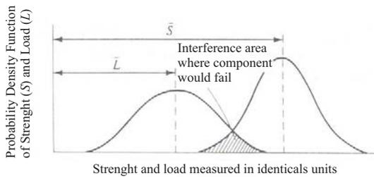
Fig. 6a: Load-strength interference diagram with interference
