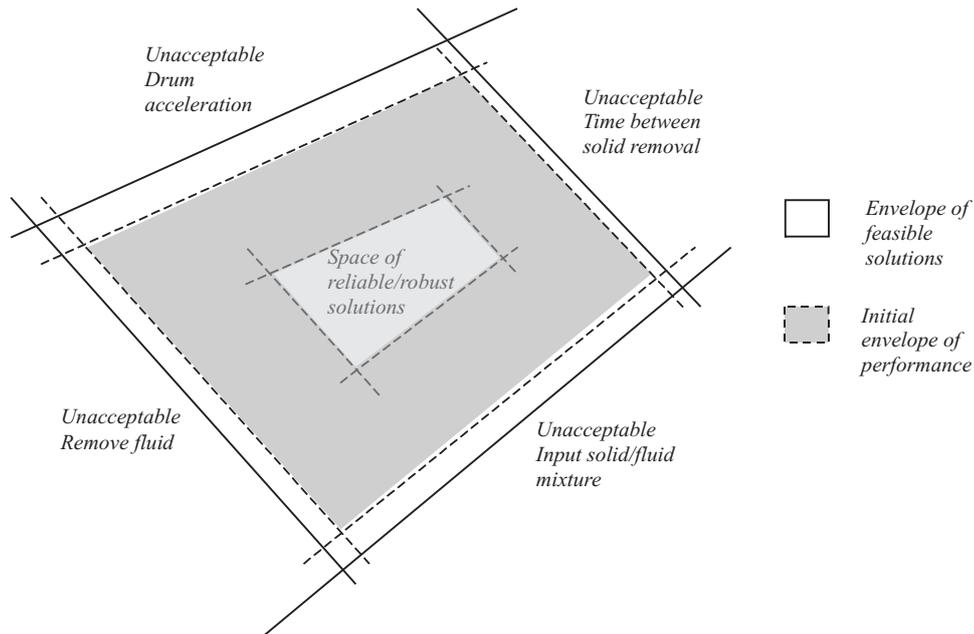
Fig. 9: Functional constraint consideration in the design space to move towards the robust solution
