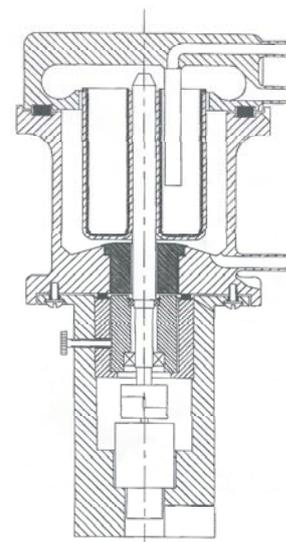
Fig. 8: Sectioned view of a conceptual centrifuge design
