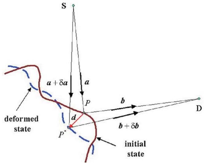
Fig. 1: Measurement of displacements
