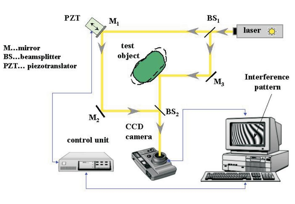
Fig. 2: Experimental scheme of the measurement system
