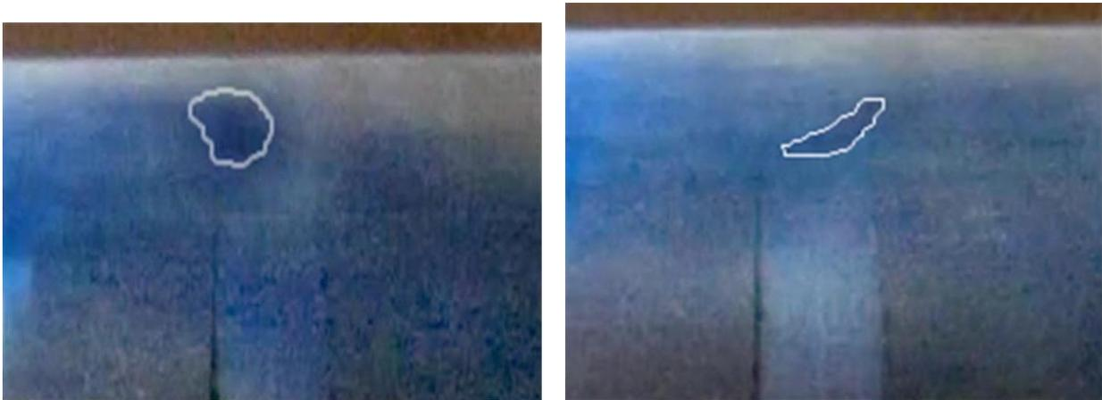
FIGURE 7. Visualisation of the flow in the grooved double pipe heat exchanger at 240 fps. (a) initial condition; (b) condition after 0.004 s.
