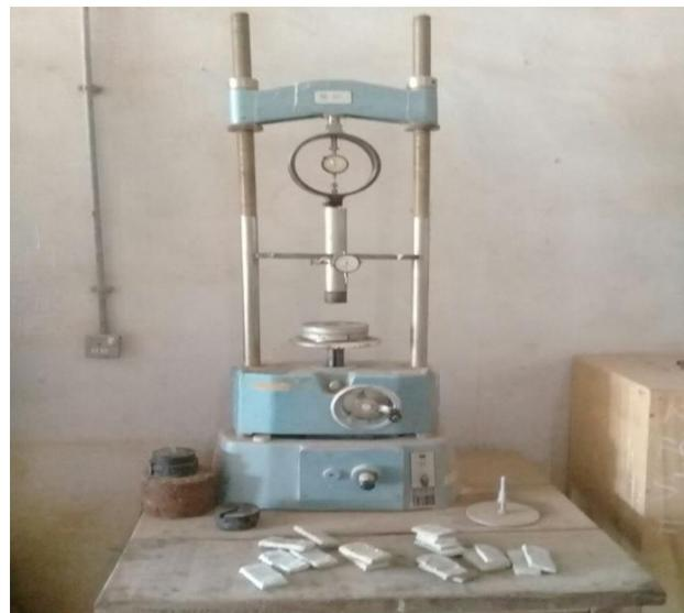
FIGURE 5. CRB CT machine (1500 kN capacity).
