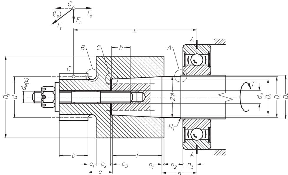
Fig. 1: Geometry of the gear wheel-shaft joint
