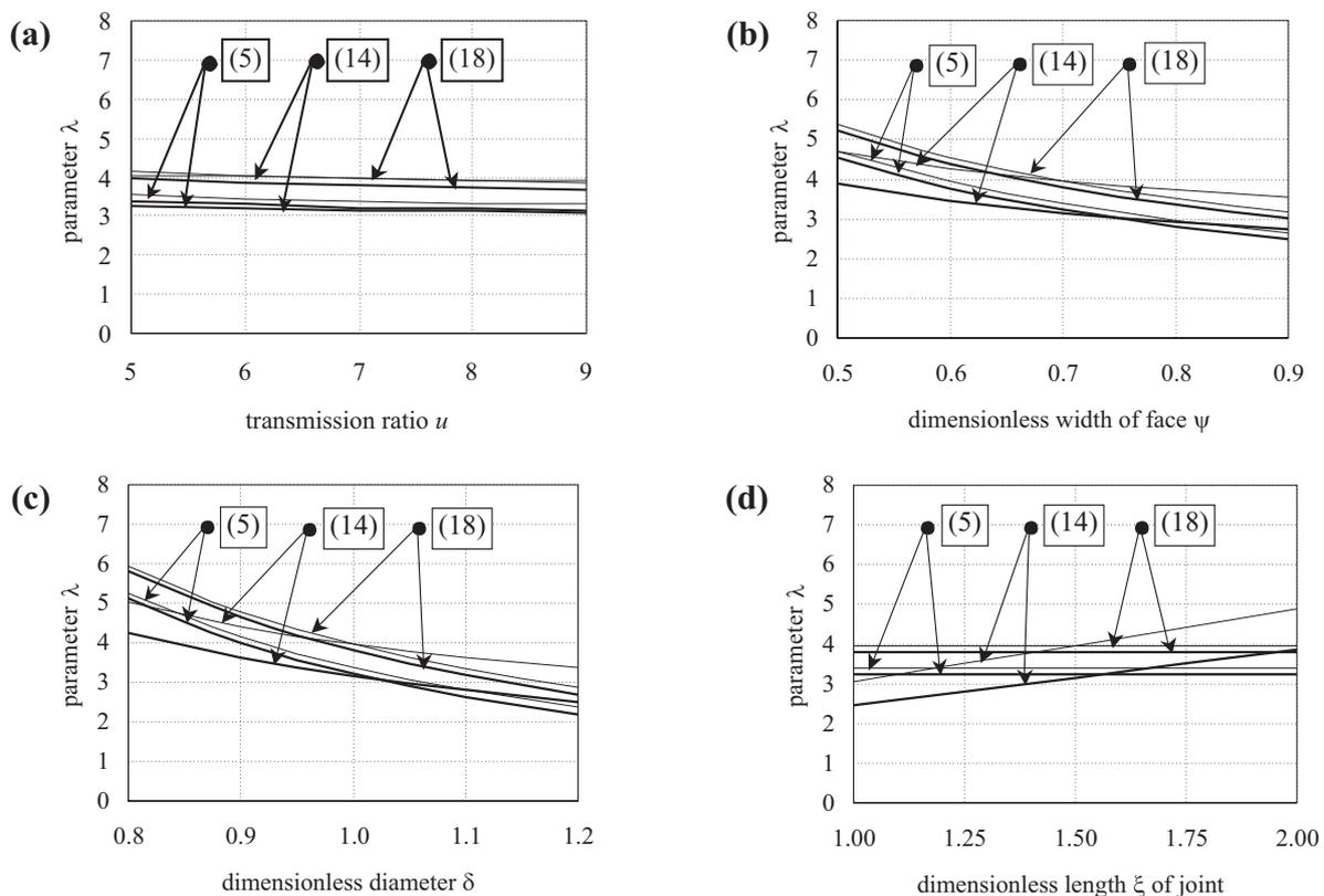
Fig. 5: Parameter  $\lambda$  versus: (a) – transmission ratio  $u$ , (b) – width of face  $\psi$ , (c) – operating pitch diameter  $\delta$ , and (d) – length  $\xi$  of the joint. Other parameters are fixed.
