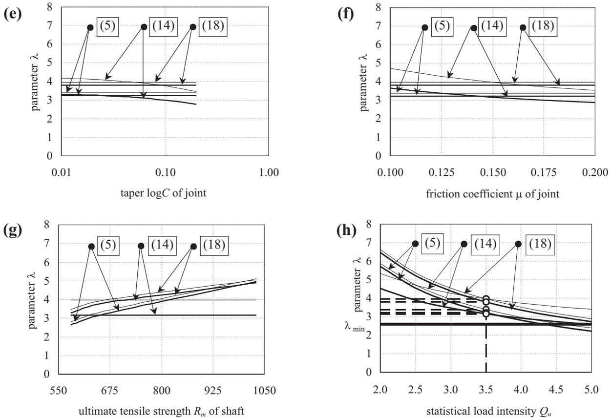
Fig. 6: Parameter  $\lambda$  versus: (e) – taper logC of the joint, (f) – friction coefficient  $\mu$  of the joint, (g) – ultimate tensile strength  $R_m$  of the shaft, and (h) – statistical load intensity  $Q_u$ . Other parameters are fixed.
