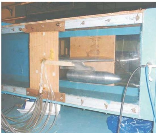
Fig. 5: Model installation inside the wind tunnel
