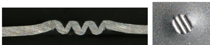
FIGURE 7. Experimental sample of grooving.
