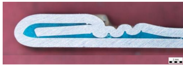
FIGURE 10. Cross-sectional view of the real hemmed sample with original dimensions (material thickness is 0.65 mm).
