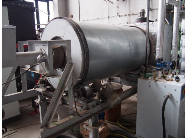
FIGURE 3. Steam rotary indirect dryer.
