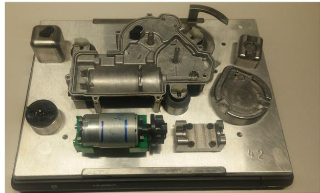
FIGURE 2. Bosch technological pallet.
