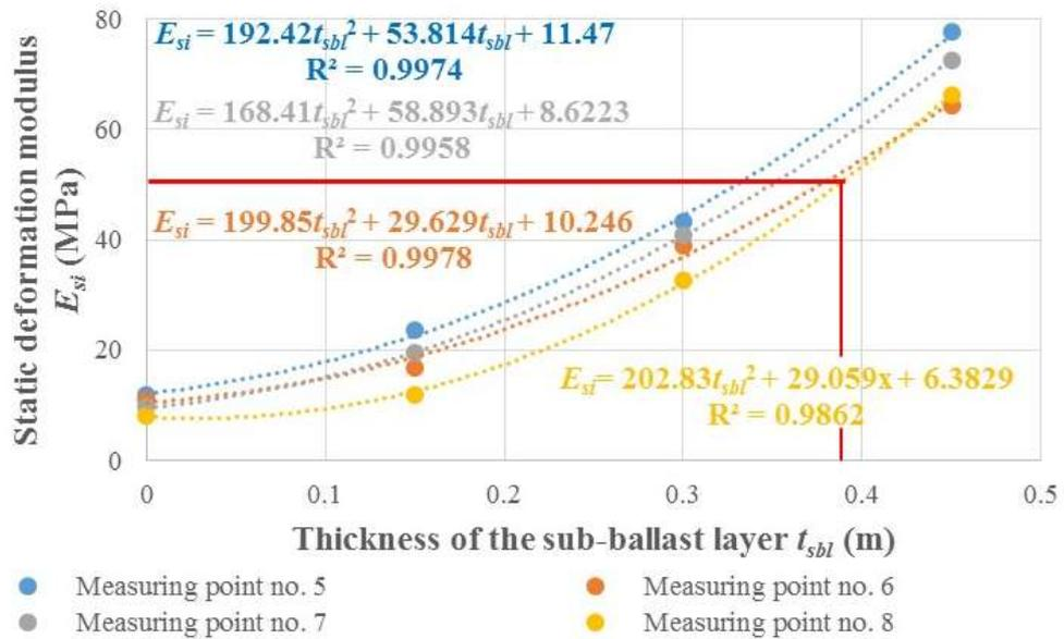
FIGURE 7. Dependence of the sub-ballast layer thickness  $t_{sbl}$  on the required value of the static modulus of deformation  $E_s$  (structure of sub-ballast layers with built-in XPS boards, low deformation resistance of the subgrade surface - approx. 10 MPa).
