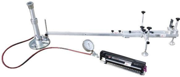
FIGURE 3. Static plate load test equipment [15].
