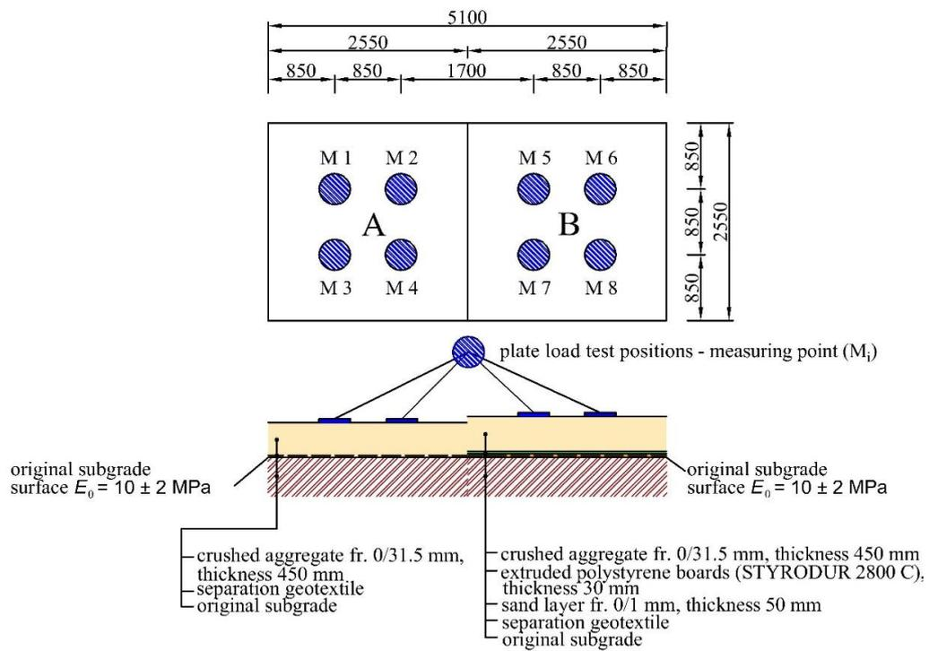
FIGURE 1. Experimental field – 1<sup>st</sup> stage of experimental measurements.
