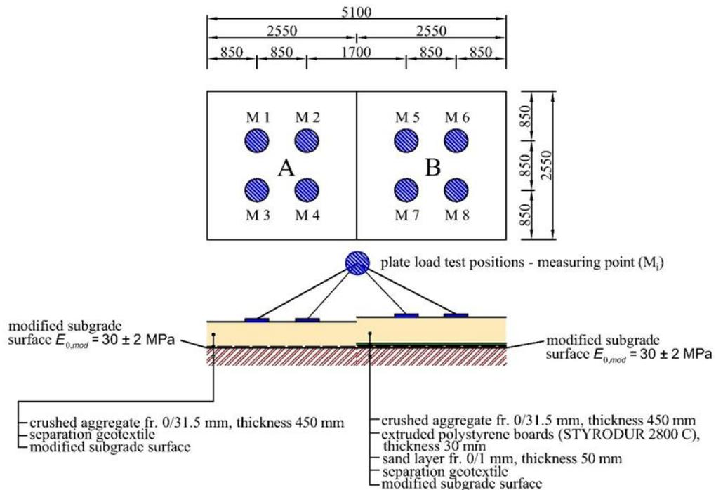
FIGURE 2. Experimental field – 2<sup>nd</sup> stage of experimental measurements.
