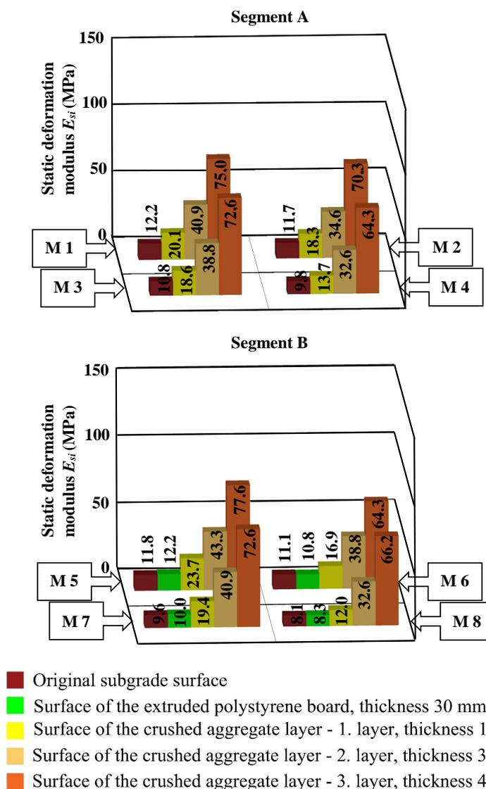
FIGURE 4. Measured values of static modulus of deformation  $E_{si}$  on the surface of individual structural sub-ballast layers - 1<sup>st</sup> stage (lower deformation resistance of the subgrade surface).
