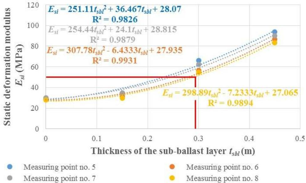
FIGURE 9. Dependence of the sub-ballast layer thickness  $t_{sbl}$  on the required value of the static modulus of deformation  $E_s$  (structure of sub-ballast layers with built-in XPS boards, higher deformation resistance of the subgrade surface - approx. 30 MPa).
