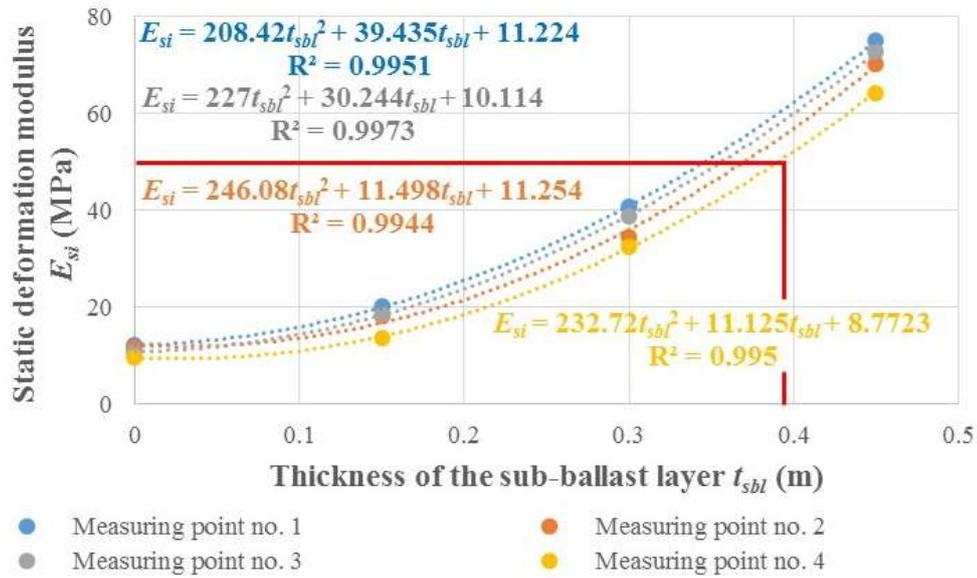
FIGURE 6. Dependence of the sub-ballast layer thickness  $t_{sbl}$  on the required value of the static modulus of deformation  $E_s$  (standard structure of sub-ballast layers, low deformation resistance of the subgrade surface - approx. 10 MPa).
