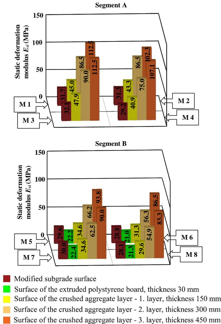
FIGURE 5. Measured values of static modulus of deformation  $E_{si}$  on the surface of individual structural sub-ballast layers - 2<sup>nd</sup> stage (higher deformation resistance of the subgrade surface).
