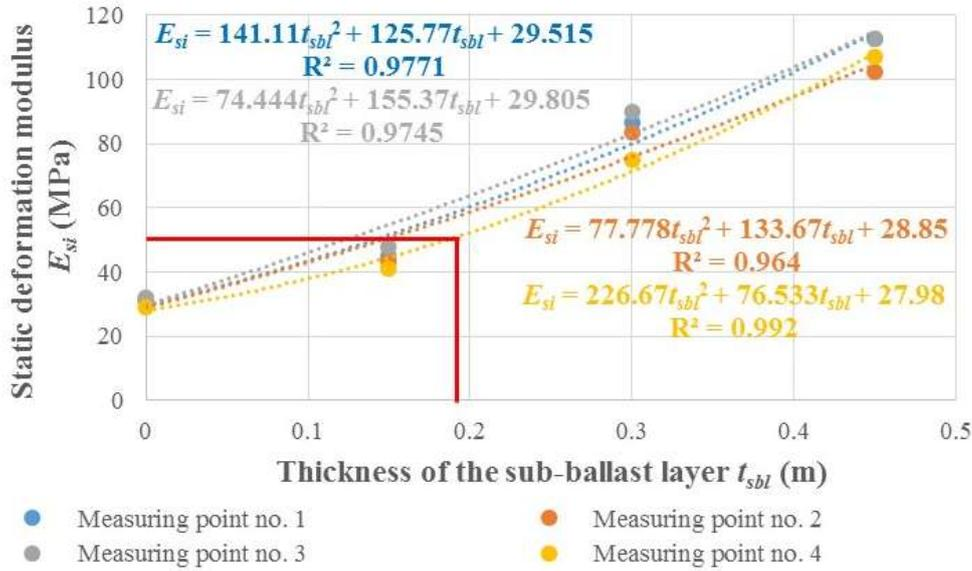
FIGURE 8. Dependence of the sub-ballast layer thickness  $t_{sbl}$  on the required value of the static modulus of deformation  $E_s$  (standard structure of sub-ballast layers, higher deformation resistance of the subgrade surface - approx. 30 MPa).
