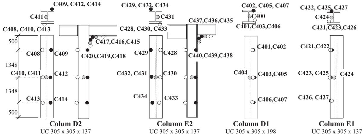
Fig. 5: Location of thermocouples on columns/beams, on flanges 20 mm from edge, on web in centreline
