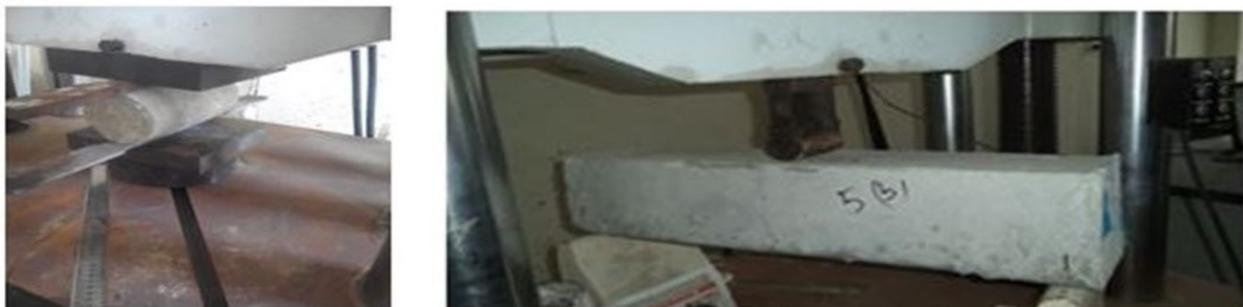
(E) . Splitting tensile strength test.
