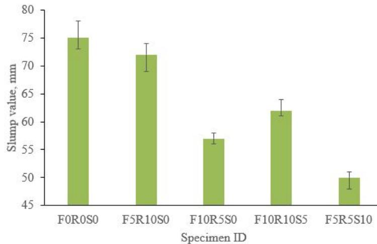
FIGURE 3. Slump value of different concrete mix.
