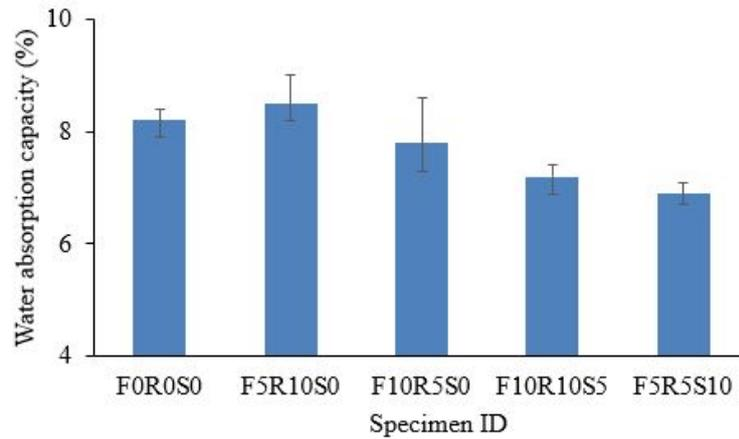
FIGURE 4. Water absorption capacity of different concrete specimens.
