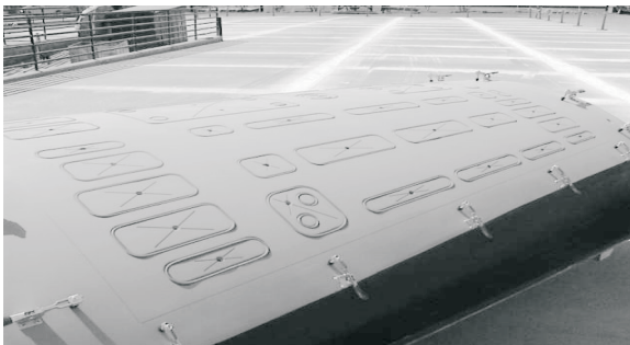
Fig. 3: Example of a vacuum specific fixture
