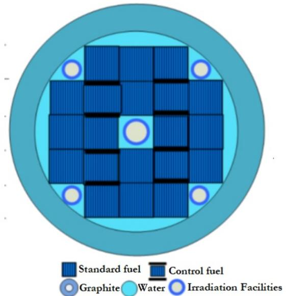
FIGURE 1. Core configuration [2].
