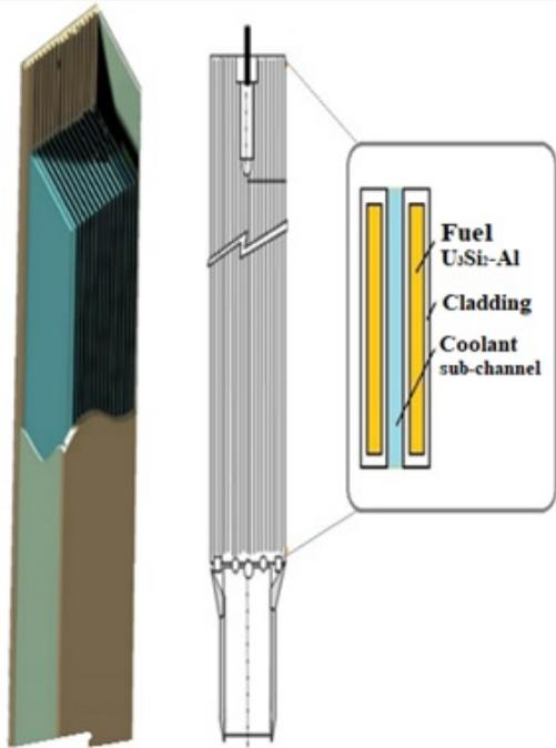
FIGURE 2. Visual representation of fuel element.
