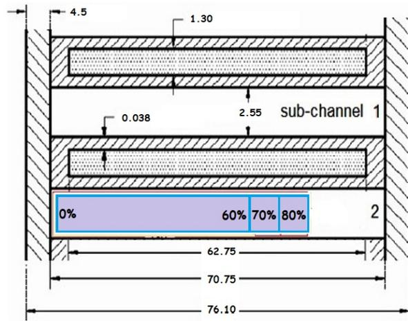
FIGURE 4. Cross-section view of sub-channel blockage simulation.
