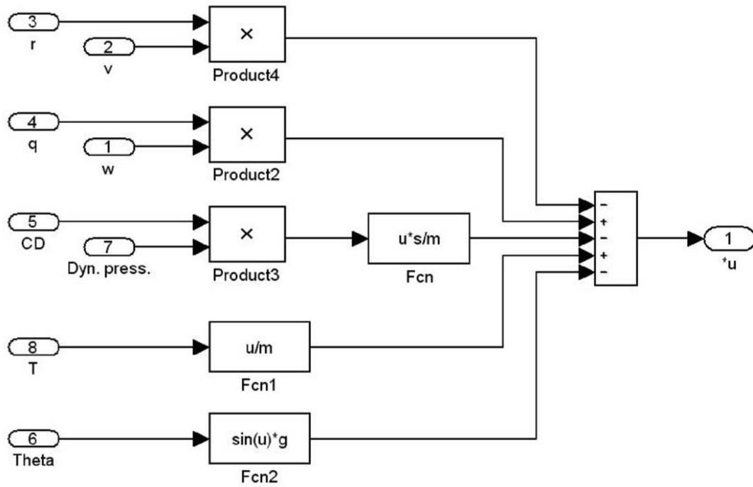
Fig. 4: Simulink<sup>®</sup> scheme representing the calculation of the first equation from Equation 1
