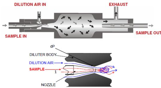
FIGURE 2. Operating principle of Dekati® dilutor [7].
