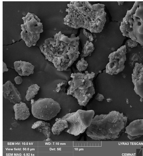
FIGURE 6. PM<sub>2,5</sub> particles captured in the impactor.
