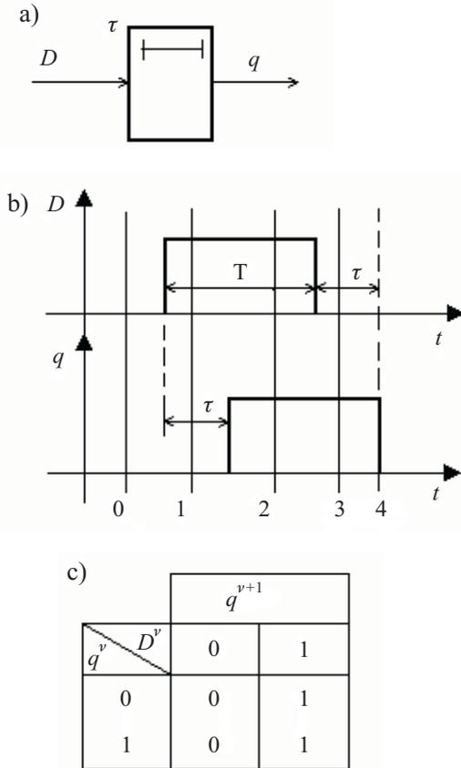
Fig. 5: a) Graphical symbol, b) action, c) delay circuit transition table
