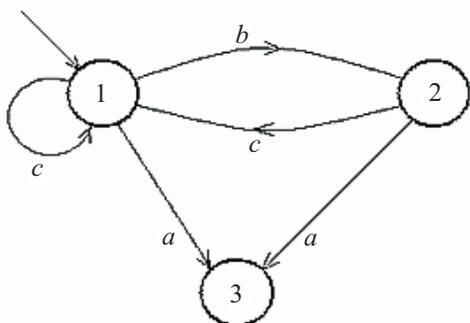
Fig. 4: Transition diagram of the automaton from Example 1
