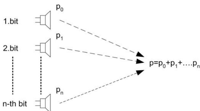
Fig. 1: Principle of a digital loudspeaker with summation of acoustic pressures
