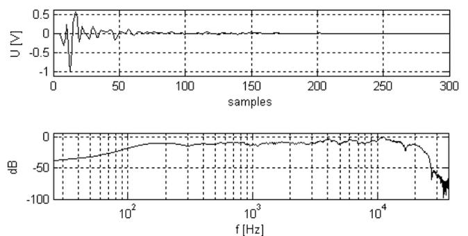
Fig. 5: Impulse and frequency response of an ARZ 6604 wide range dynamic transducer
