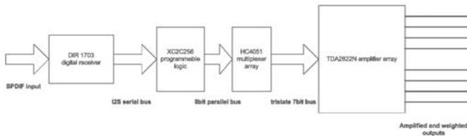
Fig. 3: Signal source chain scheme
