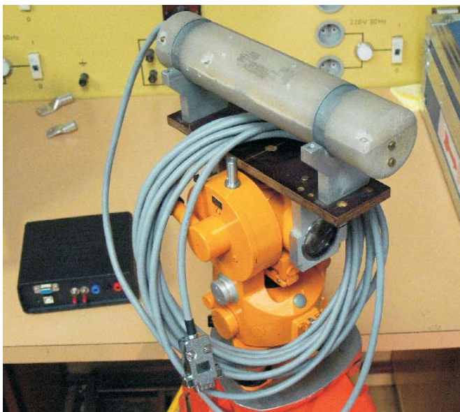
Fig. 7: Compass module on a non-magnetic tripod. On the table is a module with accumulators and a USB/serial converter
