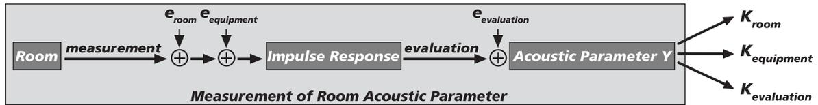
Fig. 3: Capsuled sources of measurement errors
