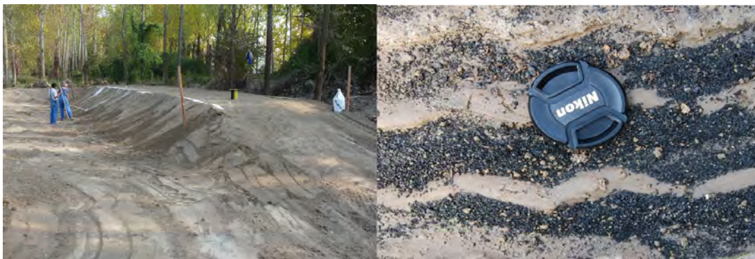
FIGURE 10. Finished test embankment (left) and the amount of coal particles (right).
