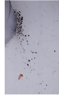
(a) Sediments after testing of CrN 2 +Cr-coated Zr-1%Nb.
