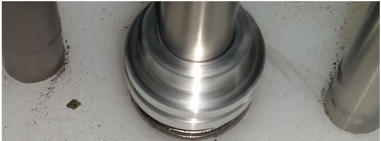
FIGURE 2. Testing equipment with 2 specimens in parallel testing: right – uncoated Zr-1%Nb; left – CrN-coated Zr-1%Nb.
