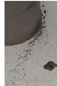
(b) Sediments after testing CrN-coated Zr-1%Nb.
