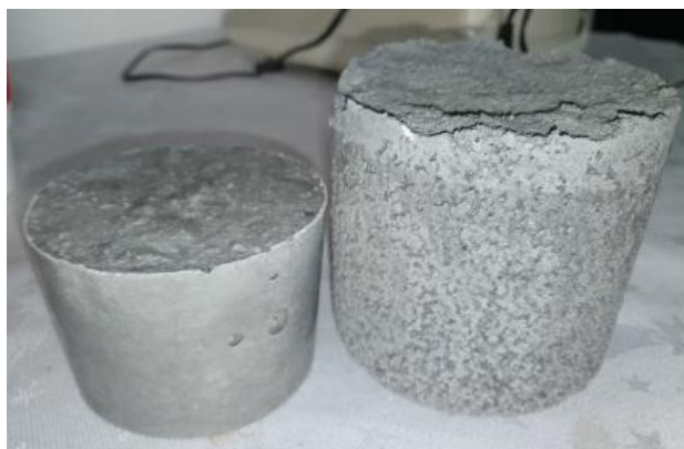
FIGURE 1. Comparison of regular (left) and careful (right) mixing of the mortar /the weight of both elements is the same/.
