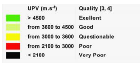
FIGURE 3. The Concrete Quality Designation (CQD) Derived from the UPV.
