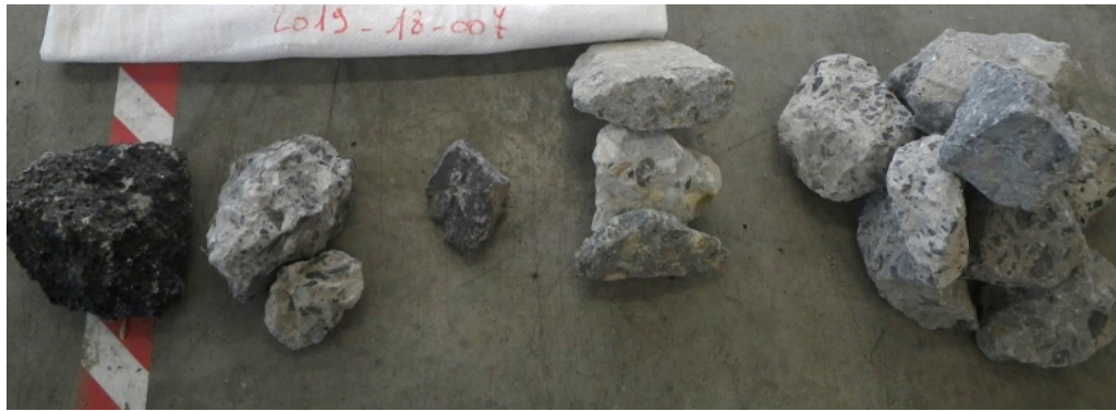
FIGURE 1. Sample 4: low quality concrete waste fraction 20-56 mm.
