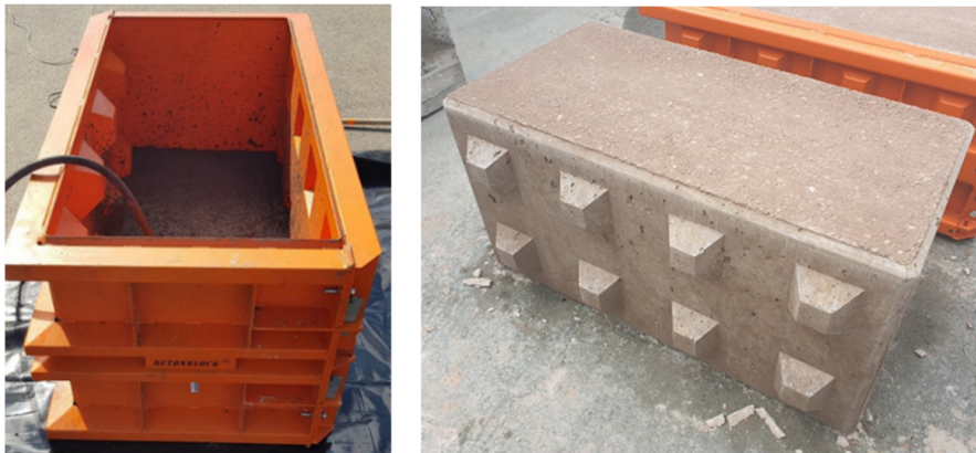
FIGURE 4. Concrete placement during the first semi-operational tests and concrete blocks.
