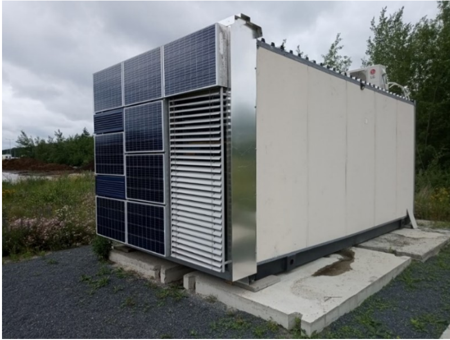
FIGURE 1. Demonstration façade curtain walling unit deployed at testing facility.
