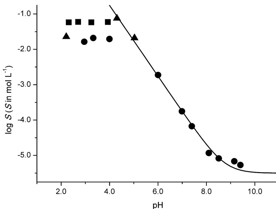
**Figure 1.** Solubility-pH profile of sibutramine according to the buffering species used in the shake-flask procedure. Legend: (●) MS-MUB, (■) hydrochloric acid (unbuffered), (▲) TFA (unbuffered).
