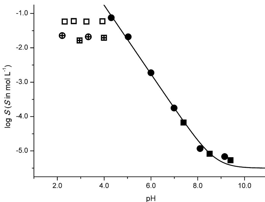
**Figure 2.** Solubility-pH profile of sibutramine according to the initial weighted solid form and the collected solid after shake-flask procedure identified by PXRD. Legend: circles and squares refer to initial species, free base or sibutramine-HCl, respectively; solid, empty, and crossed symbols indicate collected solids as free base, HCl salt, and TFA salt, respectively.
