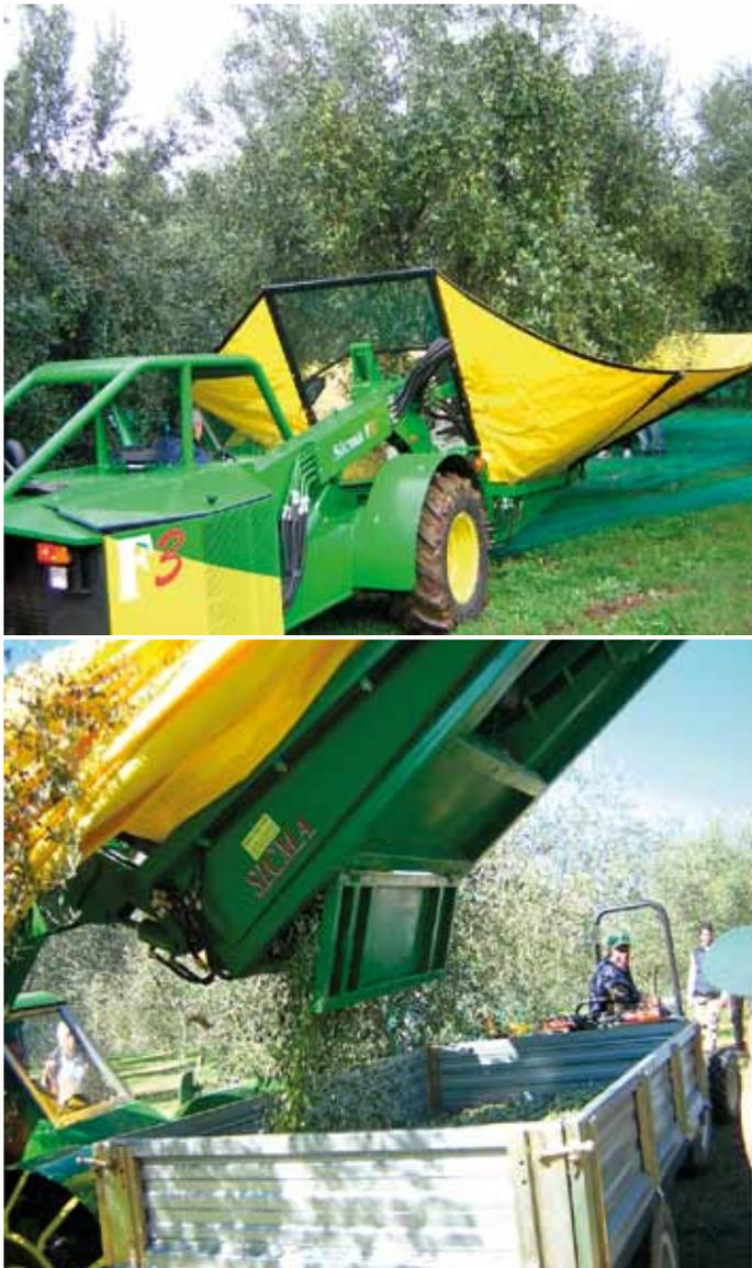
Fig. 1 - Mechanical harvesting of olives with a trunk shaker with a reversed umbrella interceptor.
