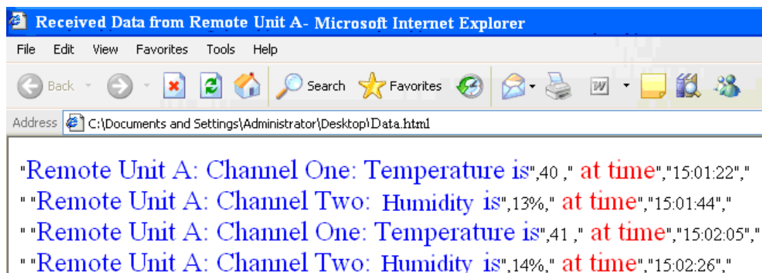
Fig.12. Received Data from Remote Unit-A Saved in HTML Page in the Master Unit.
