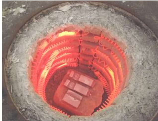
Figure (2): Assembles specimens during brazing cycle in vertical furnace.
