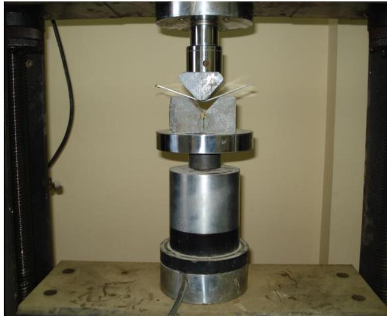
**Figure 1** The experimental setup for the V-die bending
